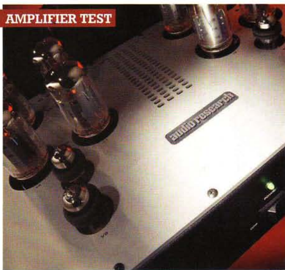
ABOVE: As an option, the alloy top-plate may be replaced by a protective tube cover which is bolted into position
